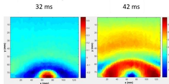
Figure 1: The shear wave propagation through the phantom at 50 Hz in 2 after 32ms and 42ms respectively
