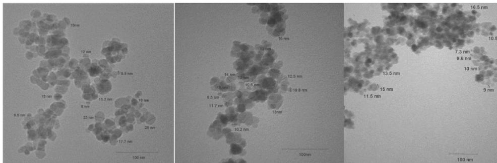
Figure 1. TEM images of Iron oxide nanoparticles for the different Latex volumes: (a)100  $\mu$ L; (b)400  $\mu$ L; (c)800  $\mu$ L
